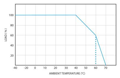
For extended service life, load should be carried in accordance with the load derating curve and to the ambient temperature derating.
